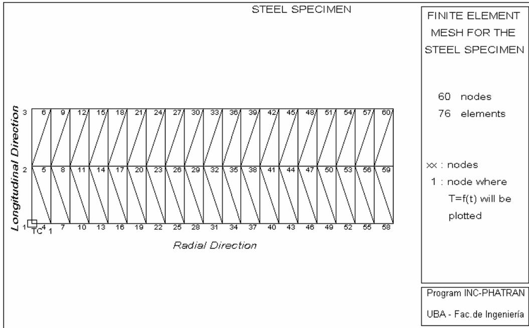
Figure 1: Finite element mesh for each of the treated samples.
