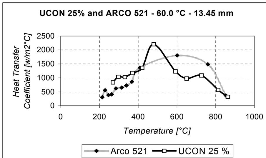
Figure 6: Heat transfer coefficient as function of temperature after mathematical simulation of samples #4 and #10. Quenching media: 25 % UCON HT and Arco 521. Sample diameter: 13.45 mm. – Quenchant temperature: 60.0 °C
