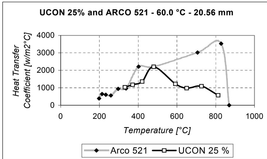
Figure 5: Heat transfer coefficient as function of temperature after mathematical simulation of samples #3 and #9. Quenching media: 25 % UCON HT and Arco 521. Sample diameter: 20.56 mm. – Quenchant temperature: 60.0 C
