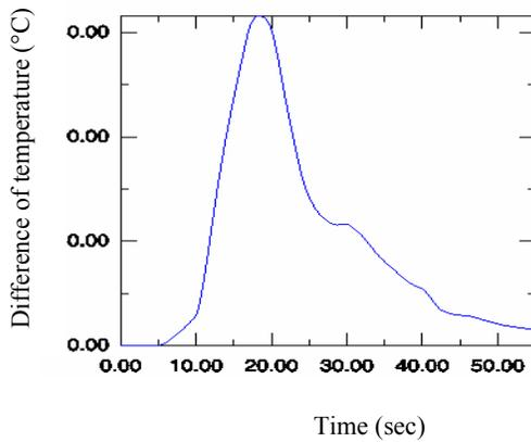
Figure 10: Difference between temperatures in the center and on the surface of sample #1.
