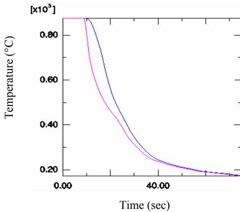
Figure 11: — : temperature on the surface of sample #11. — : temperature in the center of sample #11.
