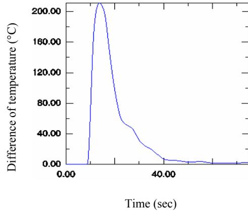
Figure 12: Difference between temperatures in the center and on the surface of sample #11.
