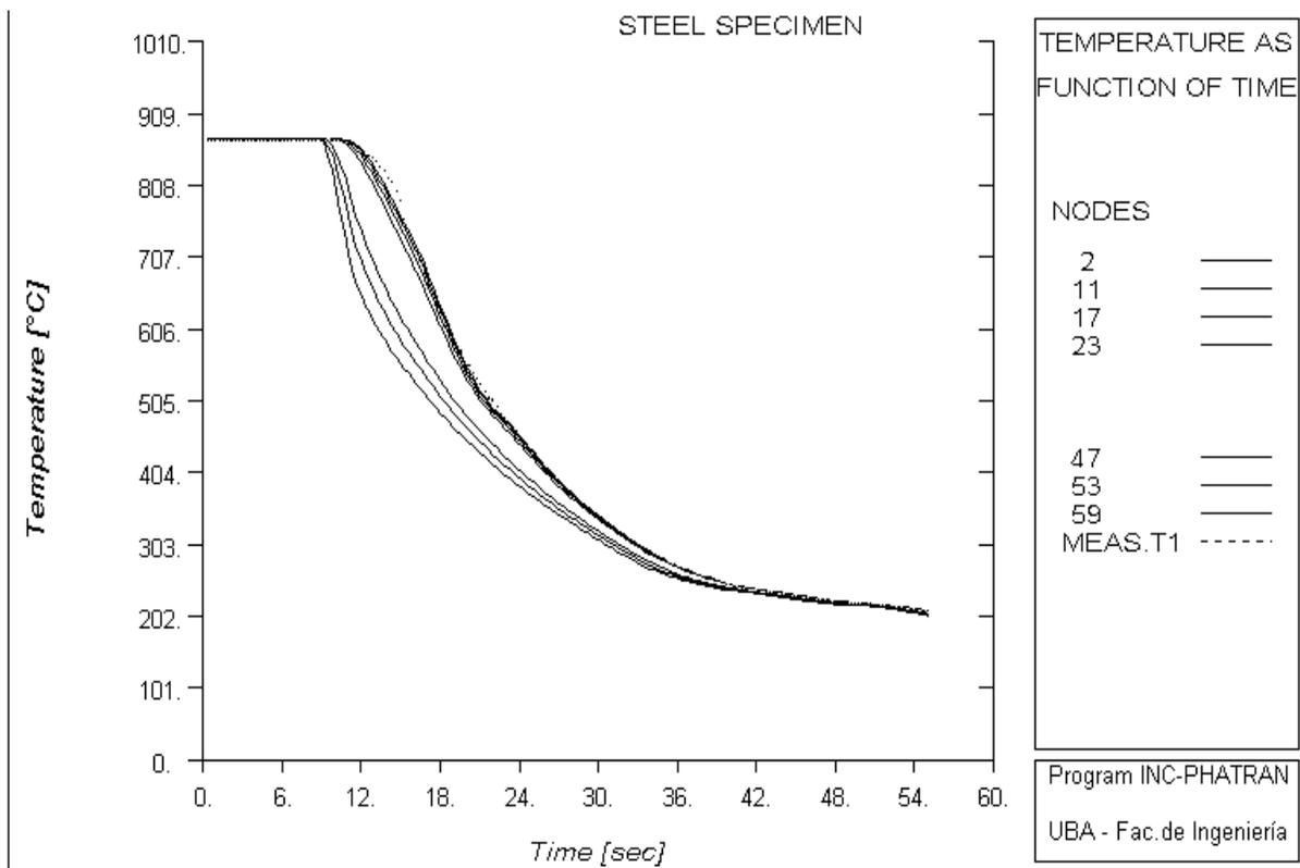
Figure 3: Measured and calculated cooling curves for sample # 11.
