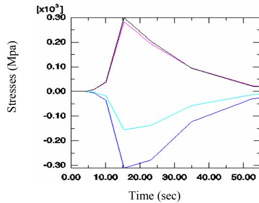
Figure 13: — :  $\sigma_z$  in the center — :  $\sigma_z$  on the surface — :  $\sigma_\theta$  in the center — :  $\sigma_\theta$  on the surface. (Sample #1).
