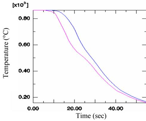
Figure 9: — : temperature on the surface of sample #1. — : temperature in the center of sample #1.
