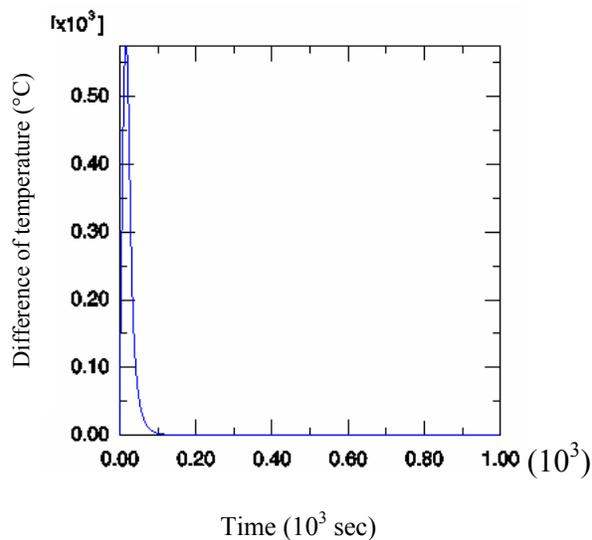
Figure 19: Difference between temperatures in the center and on the surface.
