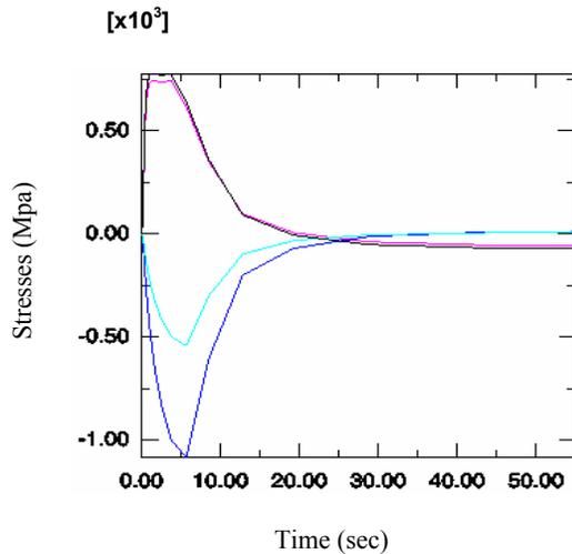
Figure 16: \_\_\_\_\_ :  $\sigma_z$  in the center \_\_\_\_\_ :  $\sigma_z$  on the surface \_\_\_\_\_ :  $\sigma_\theta$  in the center \_\_\_\_\_ :  $\sigma_\theta$  on the surface. (Sample #11).
