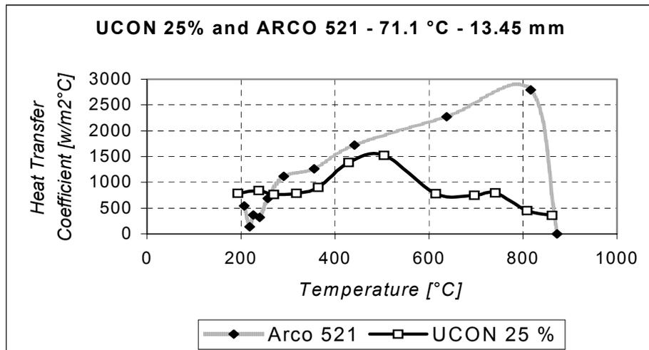
Figure 8: Heat transfer coefficient as function of temperature after mathematical simulation of samples #6 and #12. Quenching media: 25 % UCON HT and Arco 521. Sample diameter: 13.45 mm. – Quenchant temperature: 71.1 °C.
