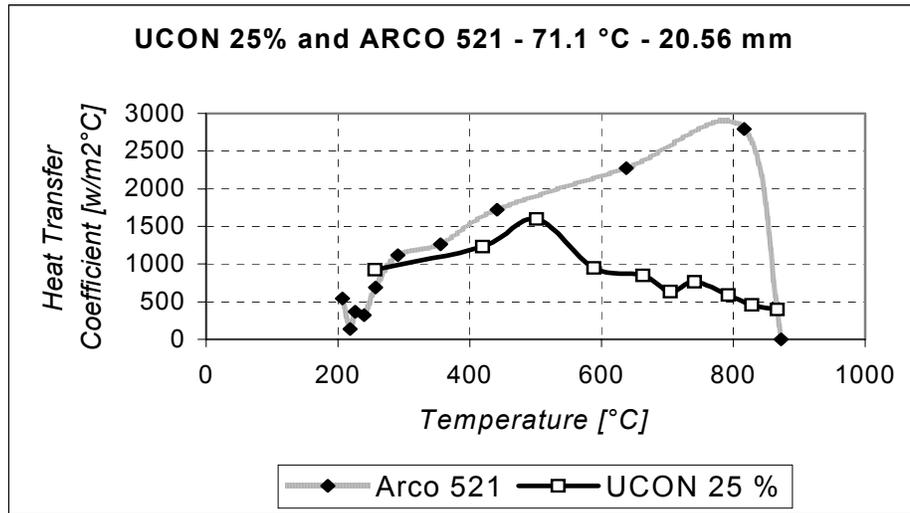
Figure 7: Heat transfer coefficient as function of temperature after mathematical simulation of samples #5 and #11. Quenching media: 25 % UCON HT and Arco 521. Sample diameter: 20.56 mm. – Quenchant temperature: 71.1 °C.
