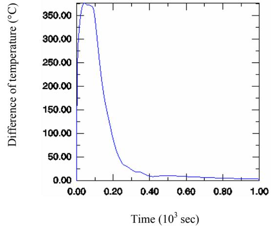
Figure 17: Difference between temperatures in the center and on the surface.
