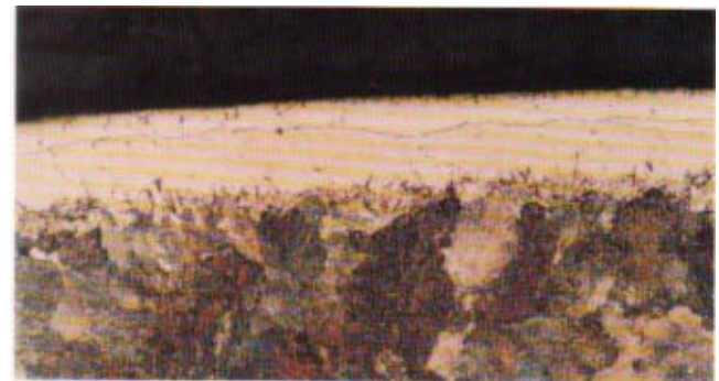
Ck 45. Austenitic Nitrocarburized @ 650°C. Dense compound zone backed by an austenite layer and nitrogen diffusion zone.
