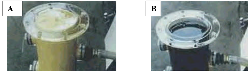
Figure 5 – Example of air bubble removal, A) aerated fluid, B) de-aerated fluid.
